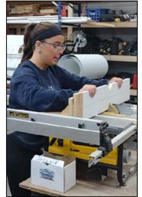
Brenna Guiliani, a sophomore and Commonwealth Honors student at Westfield State University, uses a table saw to cut a piece of wood for lattice work, which will be used on a home preservation project to restore the front porch of a historic Springfield home.
